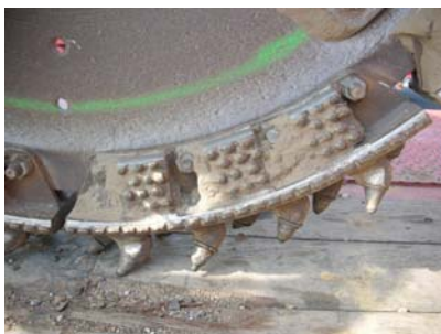
Picture 2: After a variety of different cutting jobs and 138 hours of use, the trench-cutting wheel was subjected to close inspection. (Photo: Betek)
