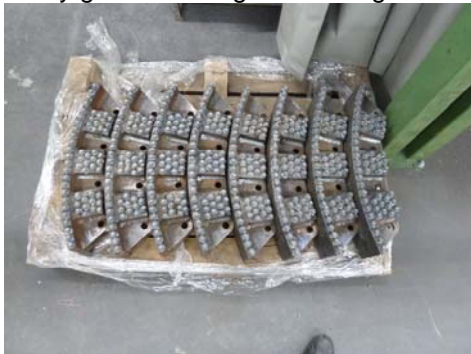
Picture 1: In order to achieve optimum protection, TungStuds were welded close together on the side of every segment of the new trench-cutting wheel. (Photo: Betek)
