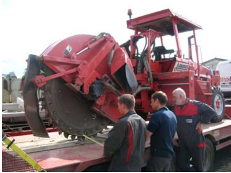
Picture 3: Well protected in this way, the cutting wheel is still 'as good as new' even after many times the usual period of use. (Photo: Betek)
