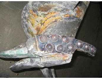
After approximately 1000 borings (secant pilewalls) with 8m depth each the TungStuds were still in good condition as you can see on the following pictures.
