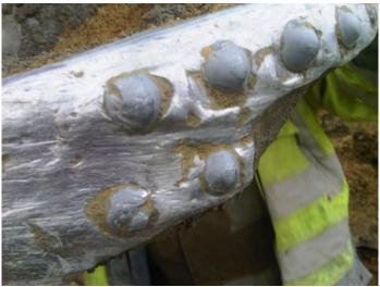
The customer was very satisfied with that test and in future he will protect the whole flights with our TungStuds BTS08 as already said, because he doubled the lifetime of his CFA's due to using TungStuds.
