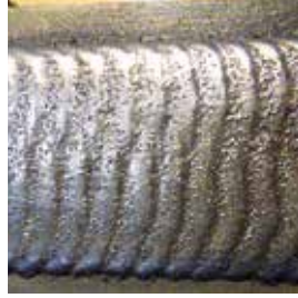
NiCr + FTC hardfacing
